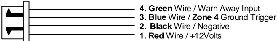
Route the red, black, blue and green wires in the 4 pin white connector from shock sensor to the control module, and plug one end into the shock sensor, and the other end into the mating orange connector on the side of the module.
