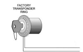
The transponders RF transmitting distance is minimal so a close fit is essential.
