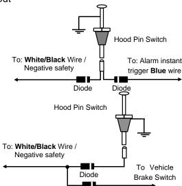
H7/6. BLACK/WHITE Wire — (-) Remote Start Enable Toggle Switch Input — (-) Neutral Safety Switch Input —
