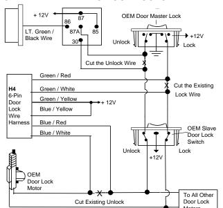
TYPICAL OF MERCEDES BENZ AND AUDI. Locate the wire under the driver's kick panel. Use the voltmeter connecting to ground, verify that you have the correct wire with the doors unlocked, the voltmeter will receive "12 volts". Lock the doors and the voltmeter wil read "0 volt". Move the alligator clip to +12V and the voltmeter will receive "12 volts". Cut this wire and make connections. Be sure to program door lock timer to 3.5 seconds. (See Feuture II - 1 Programming.)
