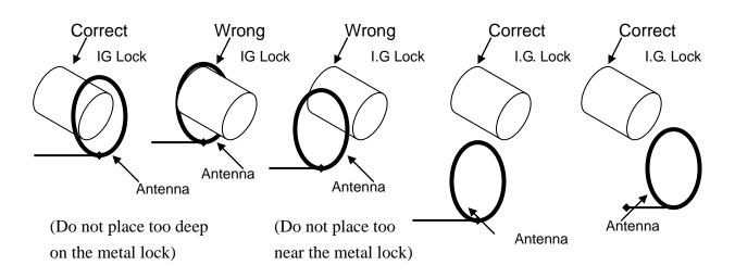
2. Antenna must be installed as an even circular shape. Do not install bended such as below:
