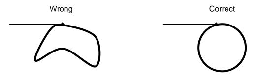
3. Please place the antenna as a 90° angle with the direction of the tag how the user usually approaches the tag's antenna to get maximum range (5 to 6 inches) as below:
