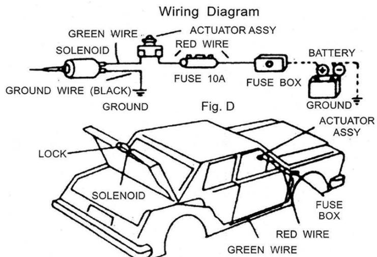
**1** Open trunk lid and find lock. Confirm "OPEN" direction of lock lever by moving the lever.
