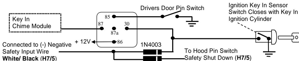
To connect to the key in sensor as shown in method 1:
