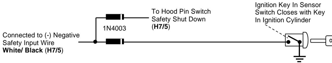
To connect to the key in sensor circuit as shown for method 2:
