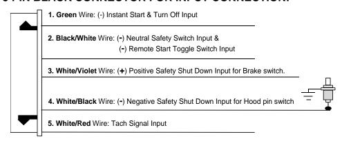
**IMPORTANT NOTE:** Directly connect the H6/2 BLACK/WHITE wire to the "GROUND" when this wire is not used.
