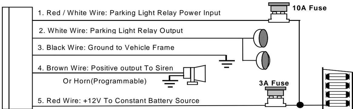
**H7: 10 PIN MINI CONNECTOR WIRE HARNESS:**
