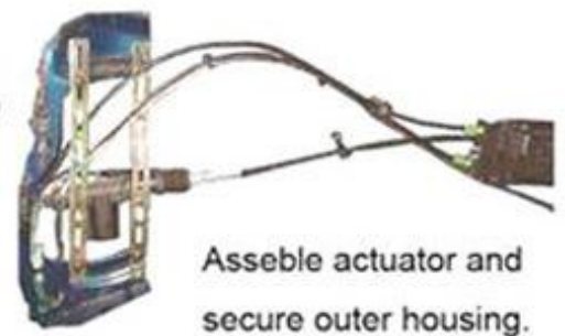
Bend hook in rod to fit actuator.
