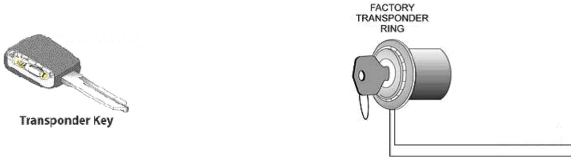
The transponders RF transmitting distance is minimal so a close fit is essential.
