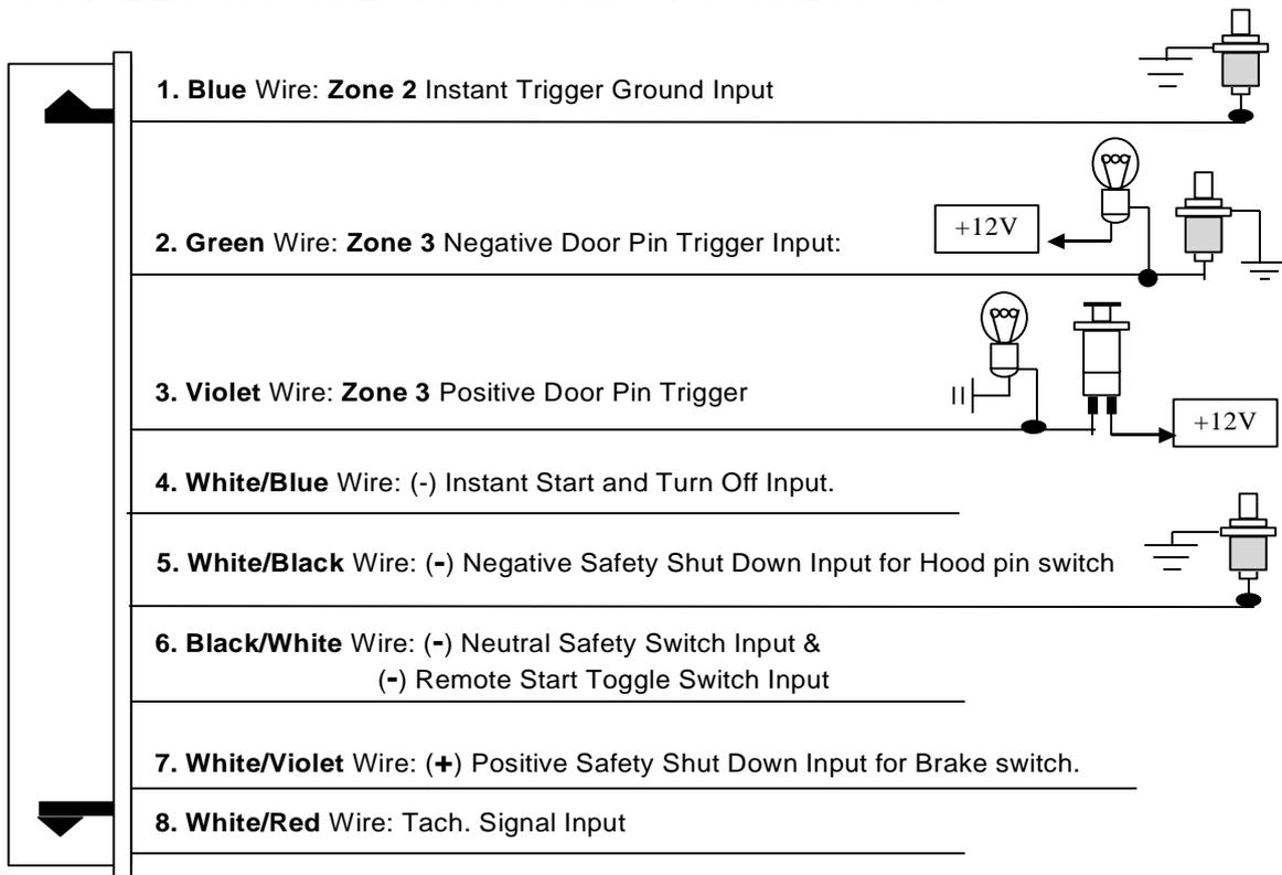
**IMPORTANT NOTE:** Directly connect the H7/6 BLACK/WHITE wire to the "GROUND" when this wire is not used.
