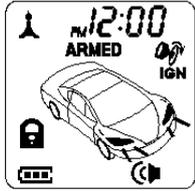
**SET** button 3 times within 3 seconds will clear the flash icon and stop melody sound on the LCD screen transmitter.
