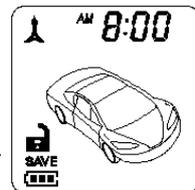
**Exit:** Press any button of the LCD remote transmitter to exit the “Power Save Mode”.
