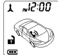
3. Turn on the ignition switch; OR press the **🔒** button to arm the system; OR press the **🔓** button to disarm the system, this outdoor driver paging function will exit.
