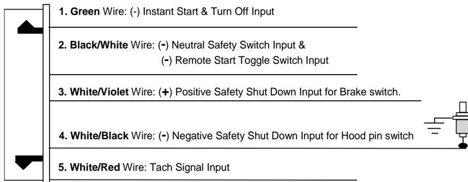
**IMPORTANT NOTE:** Directly connect the H6/2 BLACK/WHITE wire to the "GROUND" when this wire is not used.
