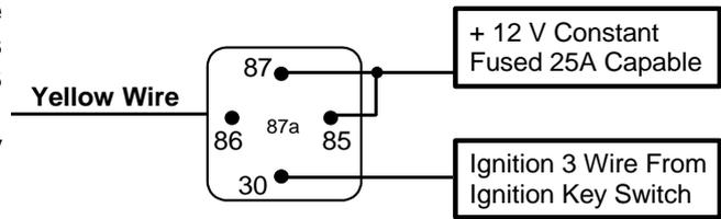
**Transponder interfacing using relay:**
