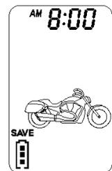
**3. Clear the Flash Icon and Melody Sound:** Press the SET button 3 times within 3 seconds will clear the flash icon and melody sound on the LCD screen transceiver
