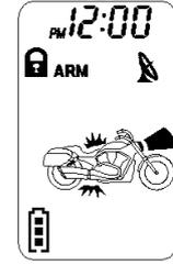
**Clear The Flash Icon And Melody Sound:** While triggering the alarm the LCD screen will alert user through melody sound and flashing trigger icon, press the SET button 3 times within 3 seconds will clear the flash icon and stop melody sound on the LCD screen transceiver.
