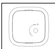
The device is usually mounted at the bottom part of the front window. In this device, there are paging (knock) sensor, which delivers the tapping impact to the Remote Control(for paging driver).
