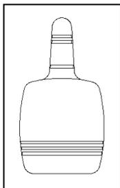
It transmits and receives RF signals with the Remote Control. If you applied optional two-way LCD screen remote transmitter on your alarm system, you must install the new two-way transceiver /Antenna module on your control module.
