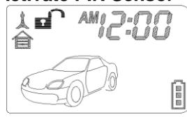
**TAMPER DISARMING:** If alarm triggered, upon disarm the system, siren chirp 4 times, parking light flash 3 times.
