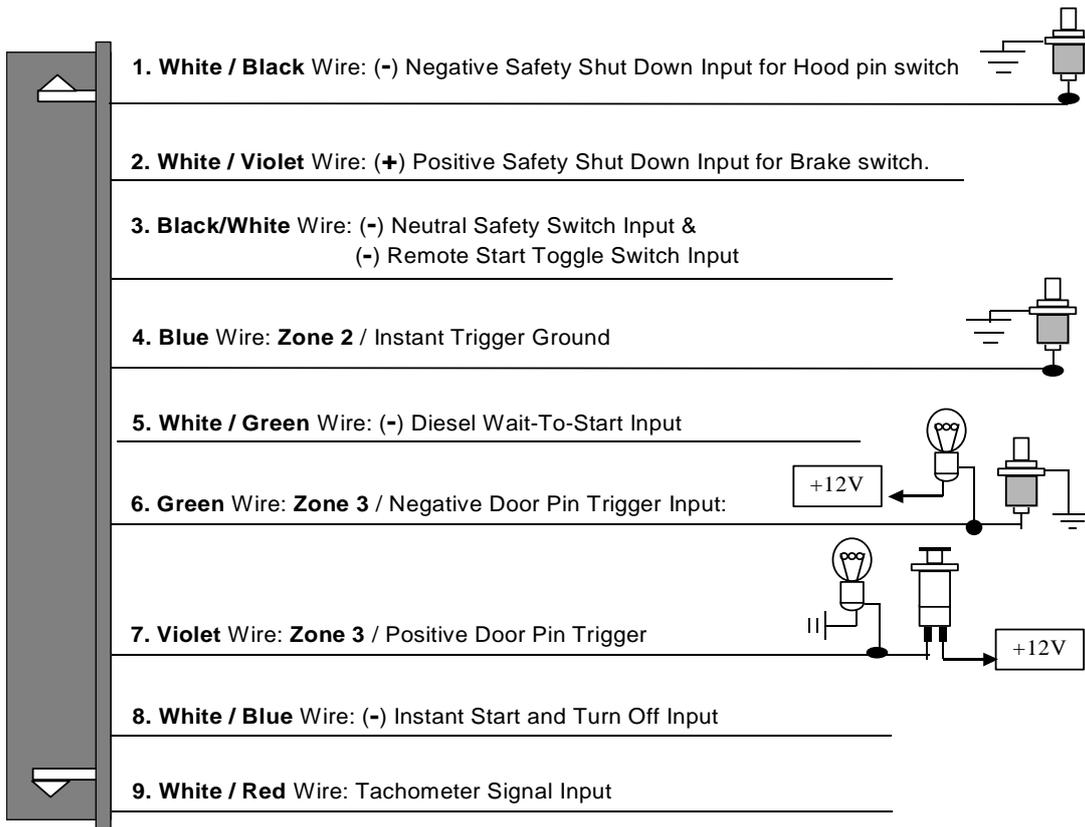
**IMPORTANT NOTE:** Directly connect the H5/3 BLACK/WHITE wire to the “GROUND” when this wire is not used.
