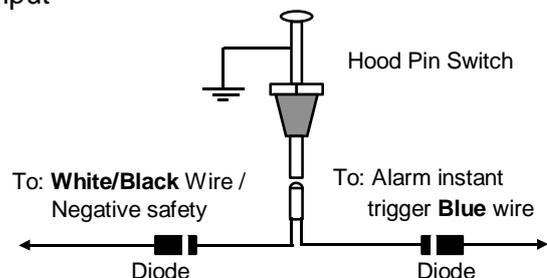
**Important!** This connection is a safety wire and must be connected as shown and tested as specified. Failure to do so may result in personal injury or property damage. See detail of wiring in the following diagram. This wire may also be used if the vehicle brake light circuit switches ground to the brake lights. An isolation diode must be used for ground switched brake light circuits and must be connected to the output of the brake switch.
