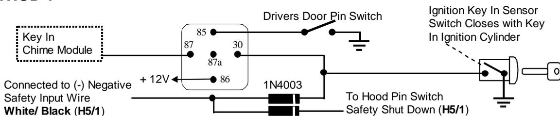
To connect to the key in sensor as shown in method 1:
