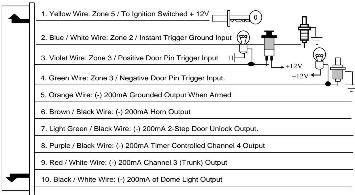
Keep wiring away from moving engine parts, exhaust pipes, and high-tension cable. Tape wires that pass through holes on the firewall to prevent frying electrical. Watch out for sharp edges that may damage wires and causes short circuit.
